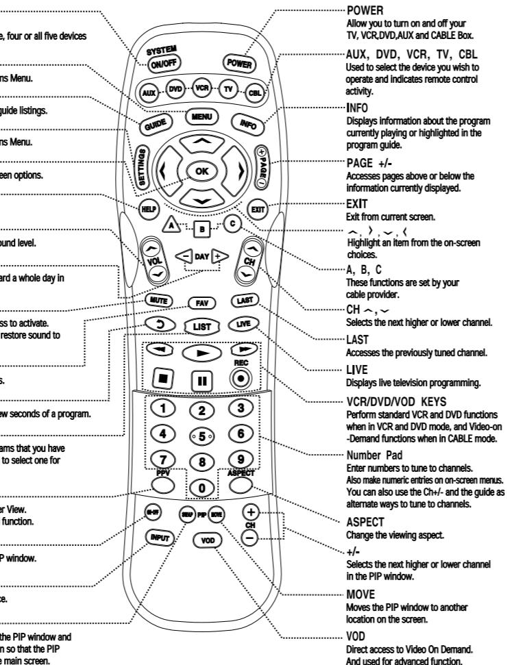
**\*Tip:** The equipment will turn off when the correct three-digit code number has been entered. You can verify you have selected the correct code by pressing the [POWER] button, the equipment should turn on or turn off.
